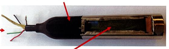
PMC fills the entire housing with a potting compound that helps to protect the electronics from water damage.
