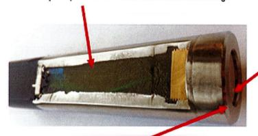
The robust ceramic sensing element is close to 60 times thicker than most oil-filled metal sensing diaphragms.
