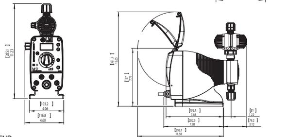
NOTE: ALL DIMENSIONS ARE IN INCHES [MM]. DIMENSIONS SHOWN ARE FOR LARGEST LIQUID END. DIMENSIONS WILL VARY DEPENDING ON LIQUID END SELECTED.
