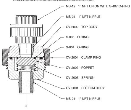
OUTLET TO E-827 EJECTOR BODY SEE A-2920/A-2922 EJECTOR ASSEMBLY DRAWING
