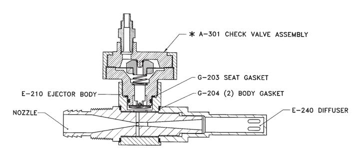
HIGH/LOW EJECTOR ASSEMBLY - MAX. 100 PPD (2000GM/HR)
