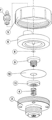
A-300S / A-320S / A-350S Low Pressure Check Valve Assembly
