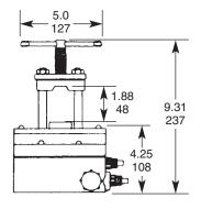
Vacuum Regulator Cylinder or Manifold Mounted\*
