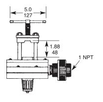
Automatic Switchover Vacuum Regulator Manifold Mounted
