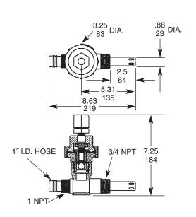
A-950 Ejector Assembly A-949 Dual Check Valve
