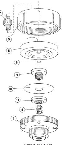
A-300/A-320/A-350 Low Pressure Check Valve Assembly
