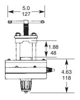
Automatic Switchover Vacuum Regulator Cylinder or Manifold Mounted\*
