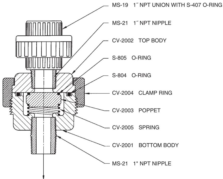
OUTLET TO E-827 EJECTOR BODY
