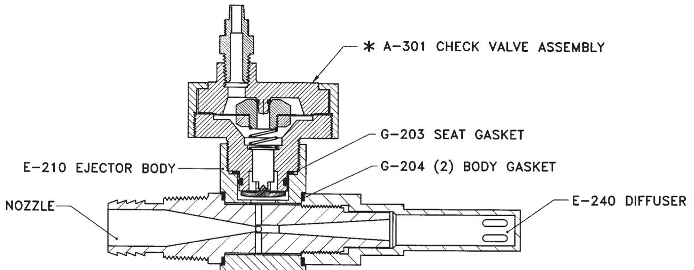
HIGH/LOW EJECTOR ASSEMBLY - MAX. 100 PPD (2000GM/HR)
