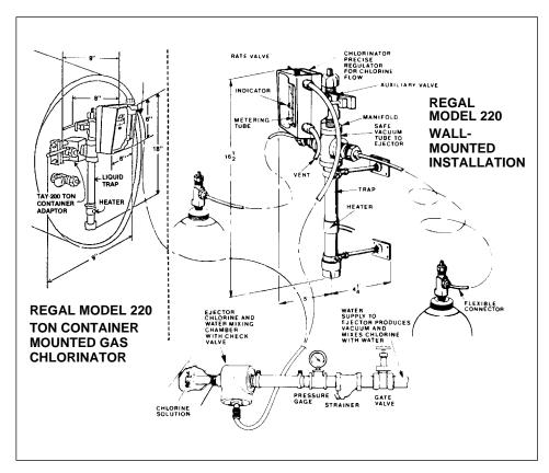
The amount of water required to operate the ejector depends upon the chlorine feed rate, water back pressure and water supply pressure available. Generally, the higher the chlorine flow and higher back pressure the greater the water flow is needed.
