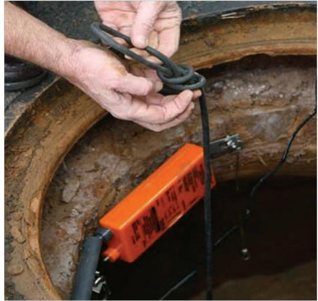
The M-80 has two float inputs on its connection wire harness. The RED and WHITE wires are the Digital Input 1 (typically the low float and called “Surcharge Alarm”) and the GREEN and BLACK wires are for Digital Input 2 (typically the higher float and called “High Level Alarm”).
