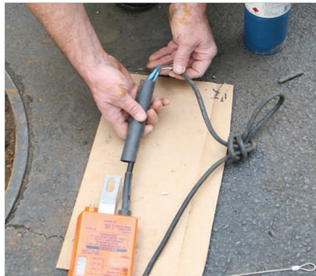
**NEVER** allow the floats to hang directly from the M-80 without using the latching support hook (carabineer). The float wire “pigtail” that exits from the M-80 **IS NOT** designed to support the weight of the hanging floats and doing so will eventually destroy the float wire seal and allow water into the M-80.
