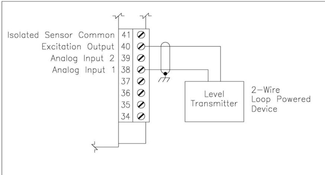
**Figure 5.3 – 2 wire, 4-20 ma Sensor Connections**
