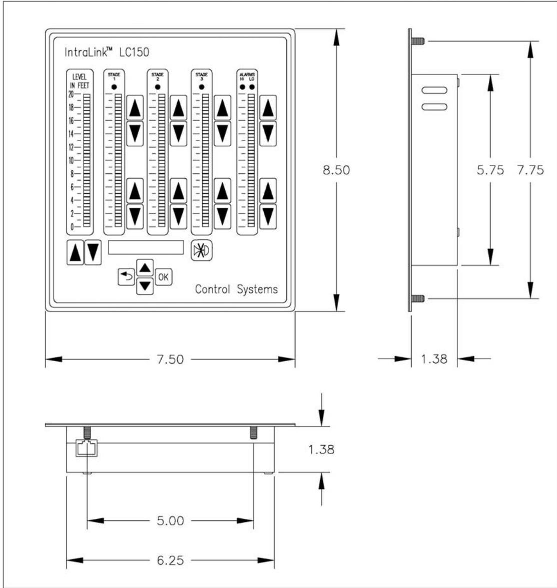
**Figure 4.3 – LC150 Operator Interface Dimensioned Drawing**
