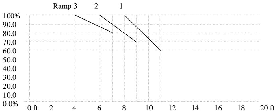
For example 2, assume the LC150 is in the Pump-Up mode with the level *above* stage-1's on setpoint (9ft) and with the following ramp and stage setpoints:
