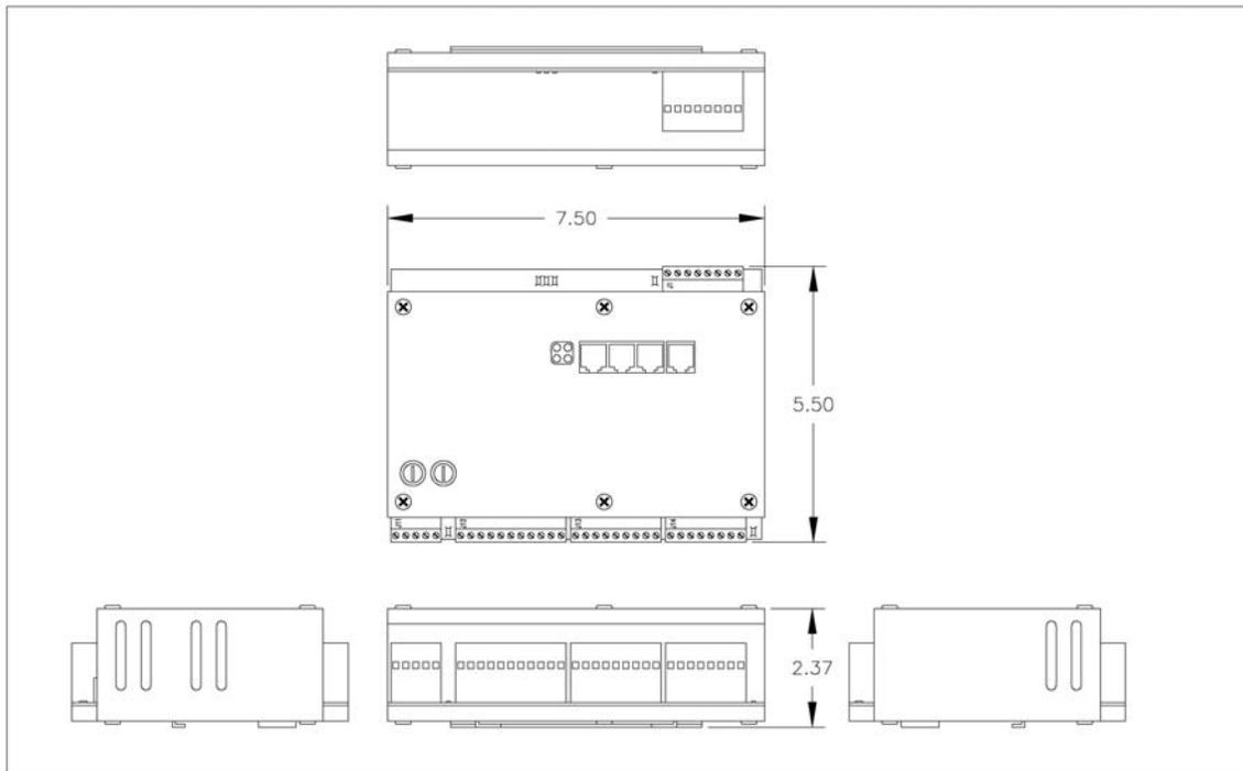
Figure 4.1 – LC150 Base Unit Dimensions
