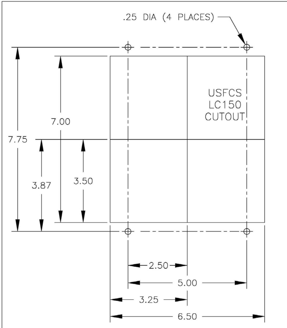
**Figure 4.2 – Door cutout Dimensions for LC150 Operator Interface**
