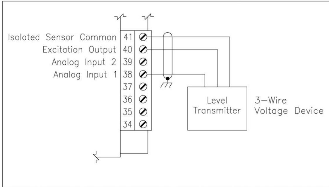
**Figure 5.5 – 3-wire Voltage Sensor Connections**
