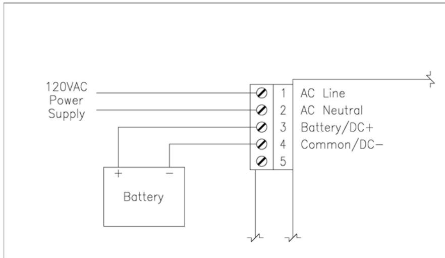
**Figure 4.4 – 120 VAC Power Connections**
