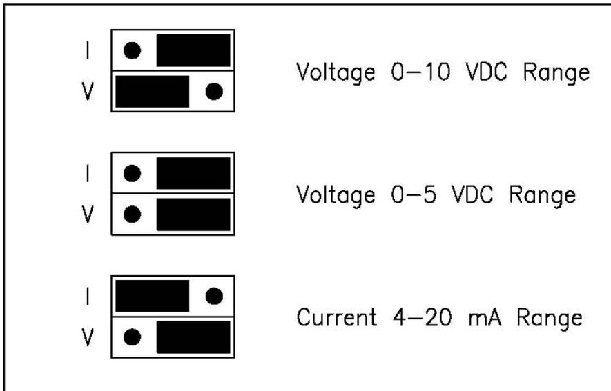
**Figure 5.2 – Analog Input Jumper Settings**
