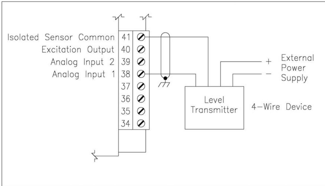
**Figure 5.4 – 4-wire, 4-20 ma Sensor Connections**
