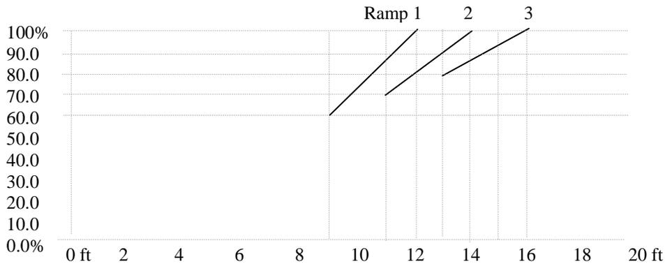
For example 1, assume the LC150 is in the Pump-Down mode with the level *below* stage-1's on setpoint (11ft) and with the following ramp and stage setpoints:
