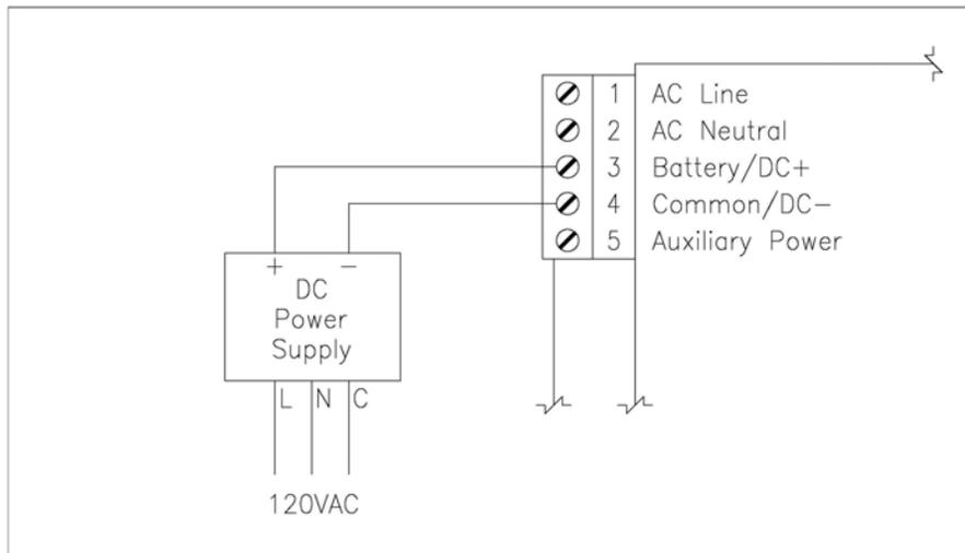
**Figure 4.5 – DC Power Connections**
