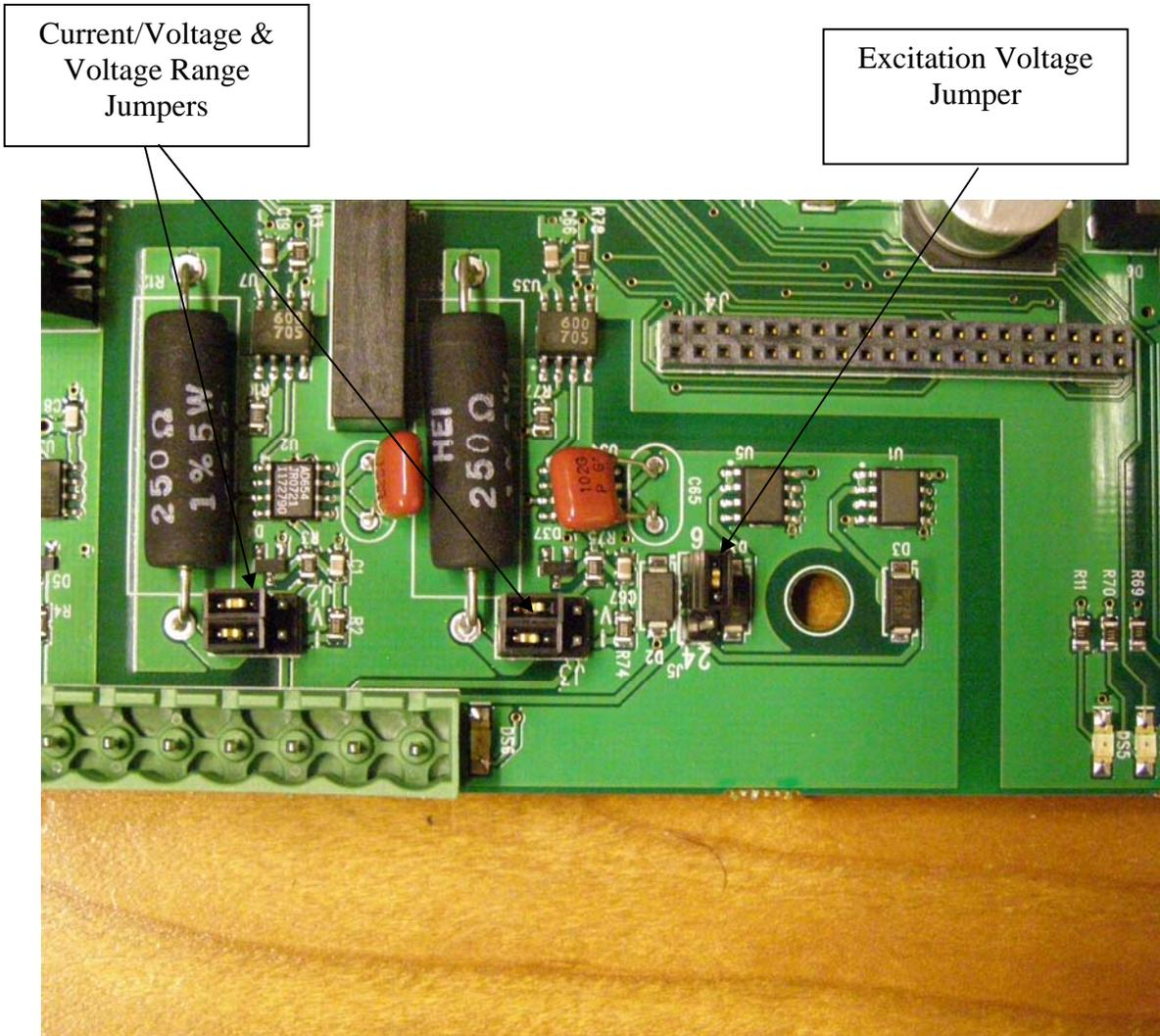
Note: The picture shows both analog inputs set for voltage operation with a 0 – 5 VDC range. The excitation voltage is set for 6 VDC. This is the default setting from the factory.
