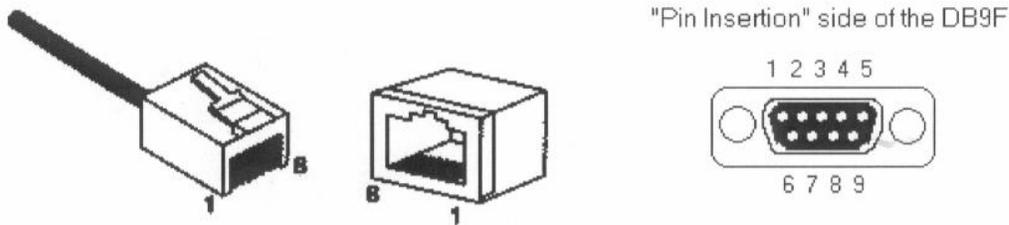
Note that when connecting the LC150 telemetry port to a CMM202C (or later), a standard “straight-through” Ethernet cable may be used. This is because the “C” version of the CMM202 includes a RJ45 jack and a jumper to connect the RTS and CTS signals. To use a standard cable, the jumper (located right behind the RJ45 connector) must be in place.
