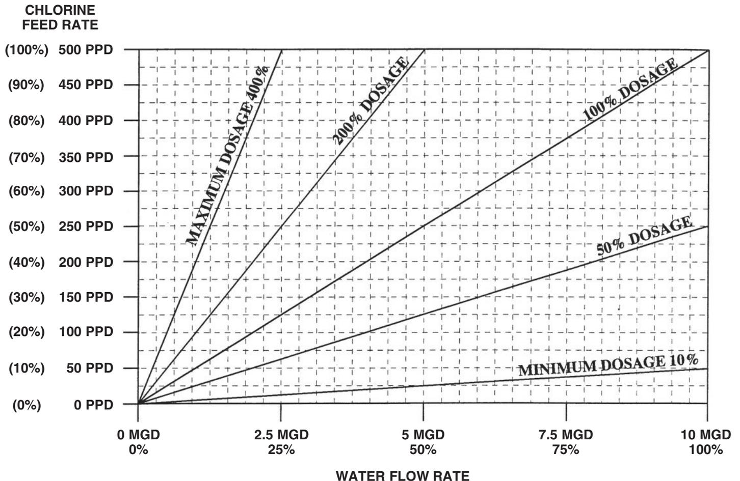
The dosage adjustment is used to set (or change) the ratio of chemical gas flow rate with respect to the process variable (Water Flow Rate) and the water quality (Demand). When using a flow proportional system, 100% dosage is achieved when the chemical feeder is operating at 100% of its feed rate based on an incoming flow meter signal representing 100% of water flow rate. As long as this ratio is maintained, the dosage is 100%.
