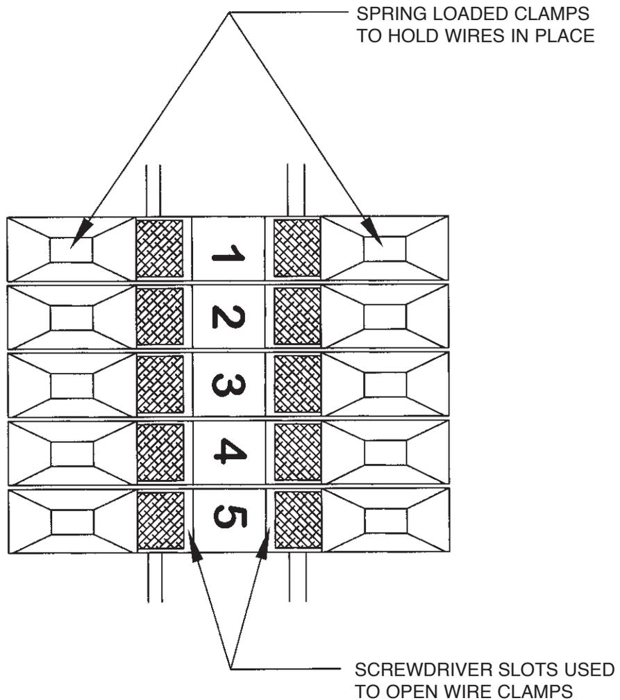
Place the blade of a small screwdriver (such as the rate valve tool supplied with your REGAL chlorinator system) into the slot and tilt the screwdriver in the direction of the terminal number. This will open the clamp and allow the wire to be inserted. Remove the screwdriver and the clamp will close to hold the wire in place.
