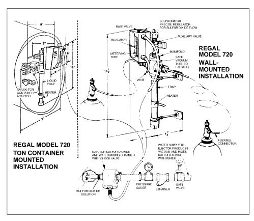
The amount of water required to operate the ejector depends upon the sulfur dioxide feed rate, water back pressure and water supply pressure available. Generally, the higher the sulfur dioxide flow and higher back pressure the greater the water flow is needed.
