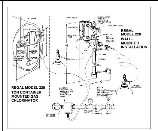
The amount of water required to operate the ejector depends upon the chlorine feed rate, water back pressure and water supply pressure available. Generally, the higher the chlorine flow and higher back pressure the greater the water flow is needed.
